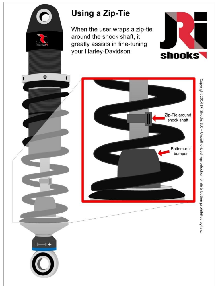
Figure 12 - Using a Zip-Tie to assist in setup
